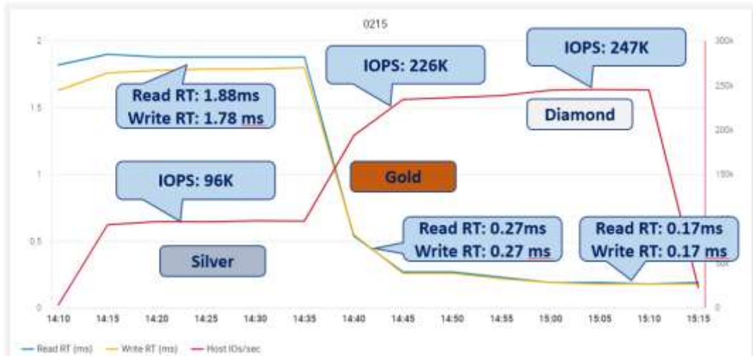
Figure 9. Single SQL Server database performance upgrade test
