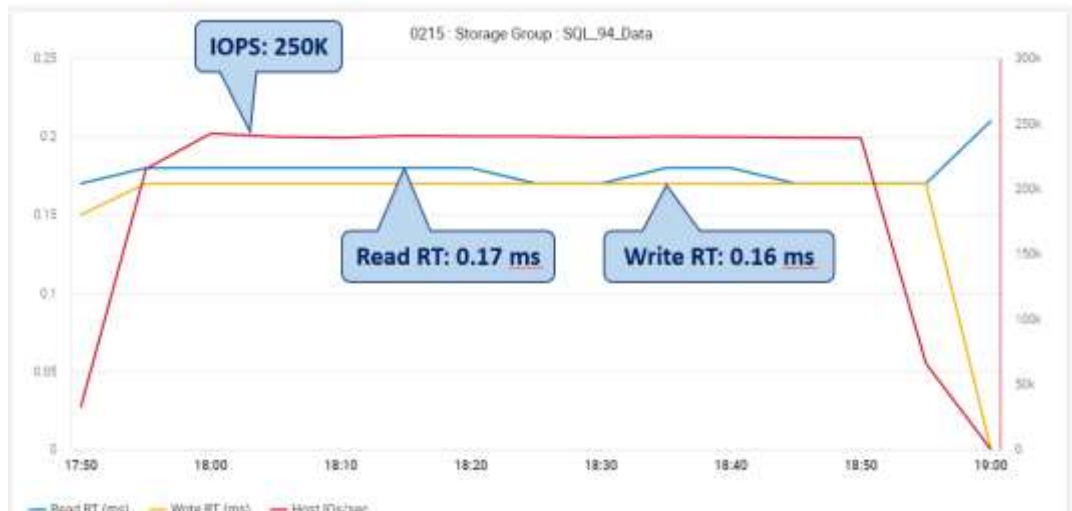
Figure 7. QoS Test for single SQL Server database
