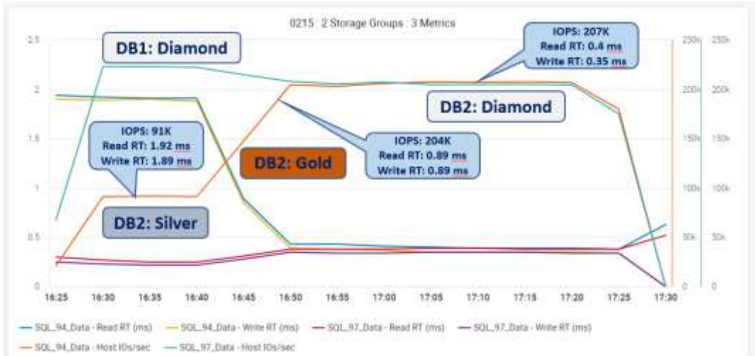
Figure 10. Onboarding application test alongside existing mission critical application
