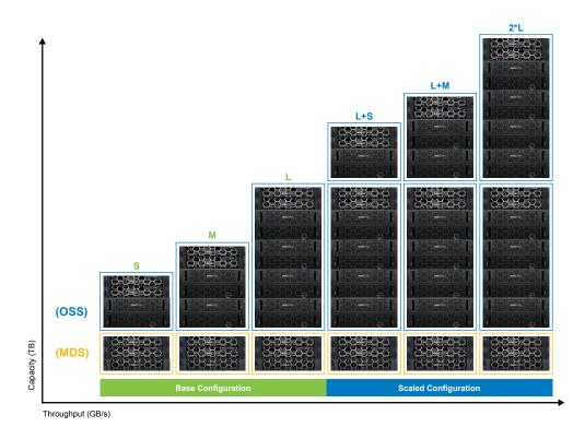
The total rack units (Total U) below represents solution sizes with metadata servers, metadata storage, object store servers and object storage with the required PowerEdge R640 management server and two networking switches.
