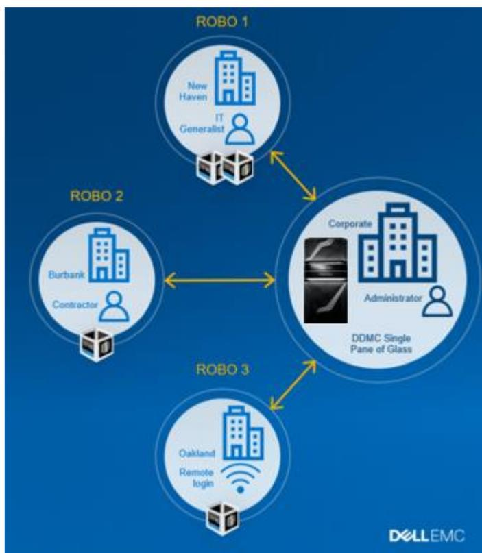
With a PowerProtect DD appliance at the main data center and a DDVE at each branch office, you get the assurance that your data at these branch offices is protected. The entire data protection environment can be managed centrally with DDMC. If a branch office has a failure or must shut down, you have the peace of mind that the protected data is not lost. DDVE will divert that data into another remote office or stores it on-premises.
