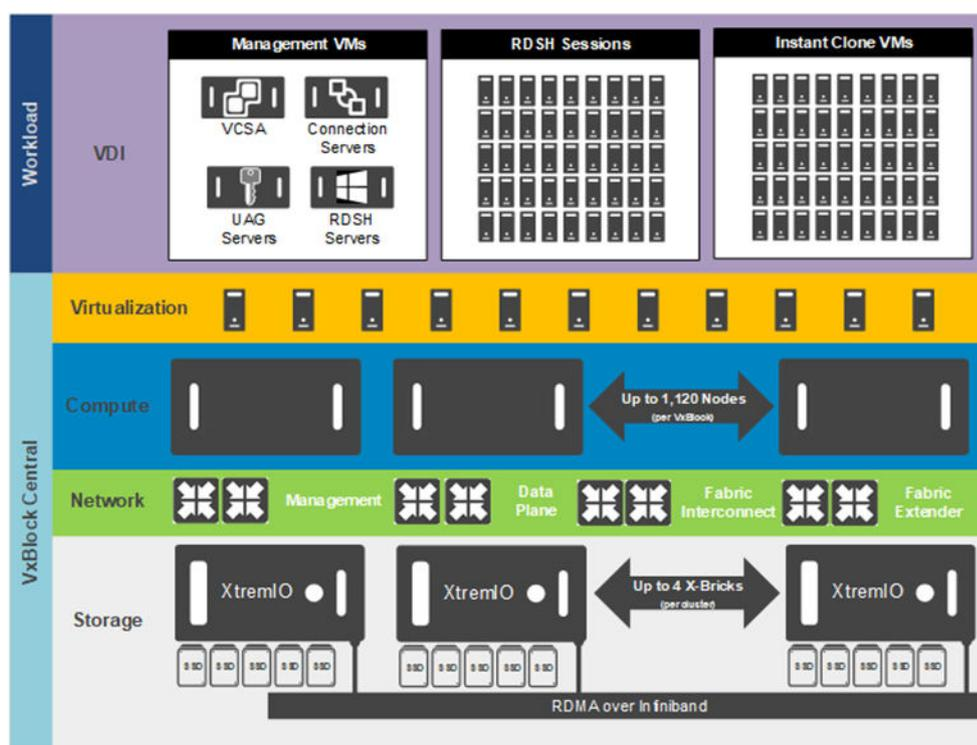
Deployment of this Ready Architecture supports all VMware cloning techniques, including full, linked, and instant cloning.
