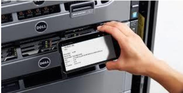
Figure 1 An administrator using iDRAC Quick Sync
