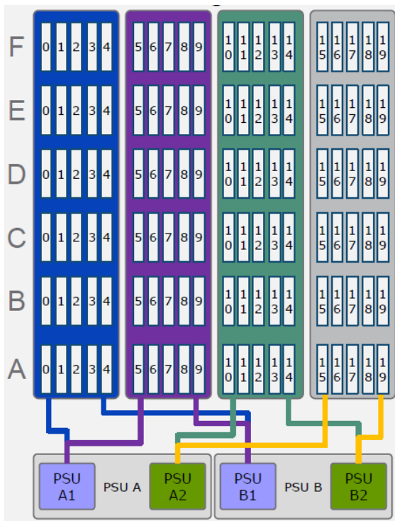
Figure 5 VMAX 950F DAE Layout – drive slots and power zones
