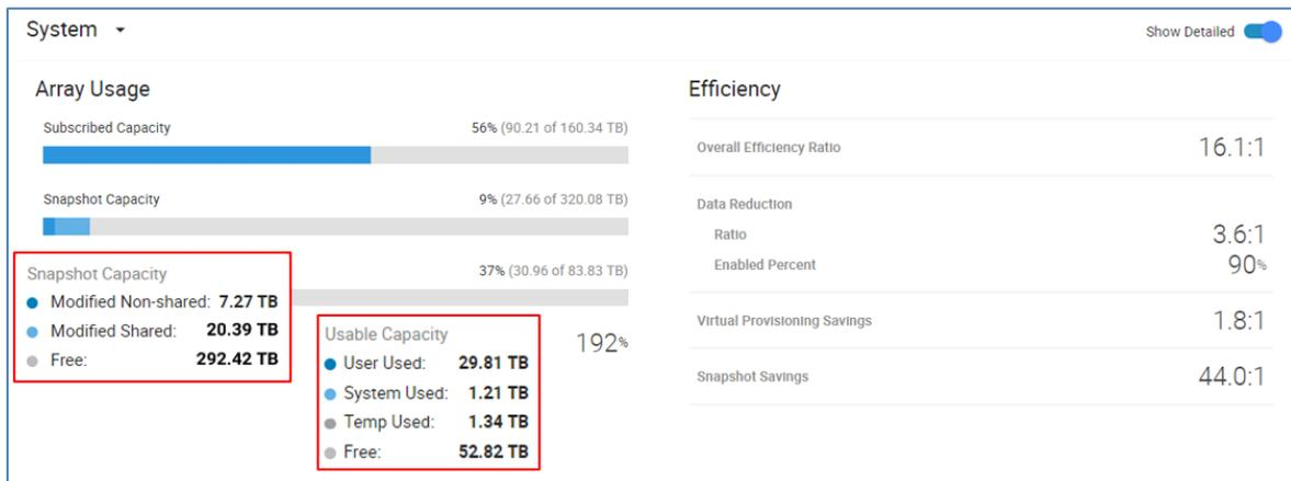
Figure 3 System Efficiency report detailed view as seen in Unisphere for PowerMax
