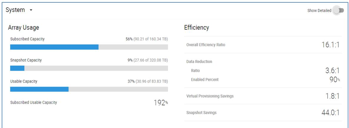
Figure 2 System efficiency report as seen in Unisphere for PowerMax
