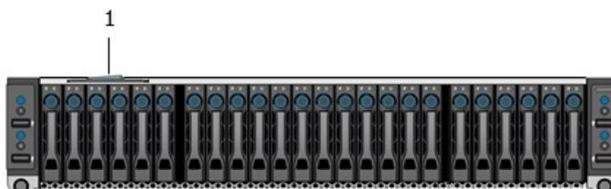
**Figure 2** VxRail Appliance product serial number tag (PSNT) location (Models 60 through 280) (continued)
